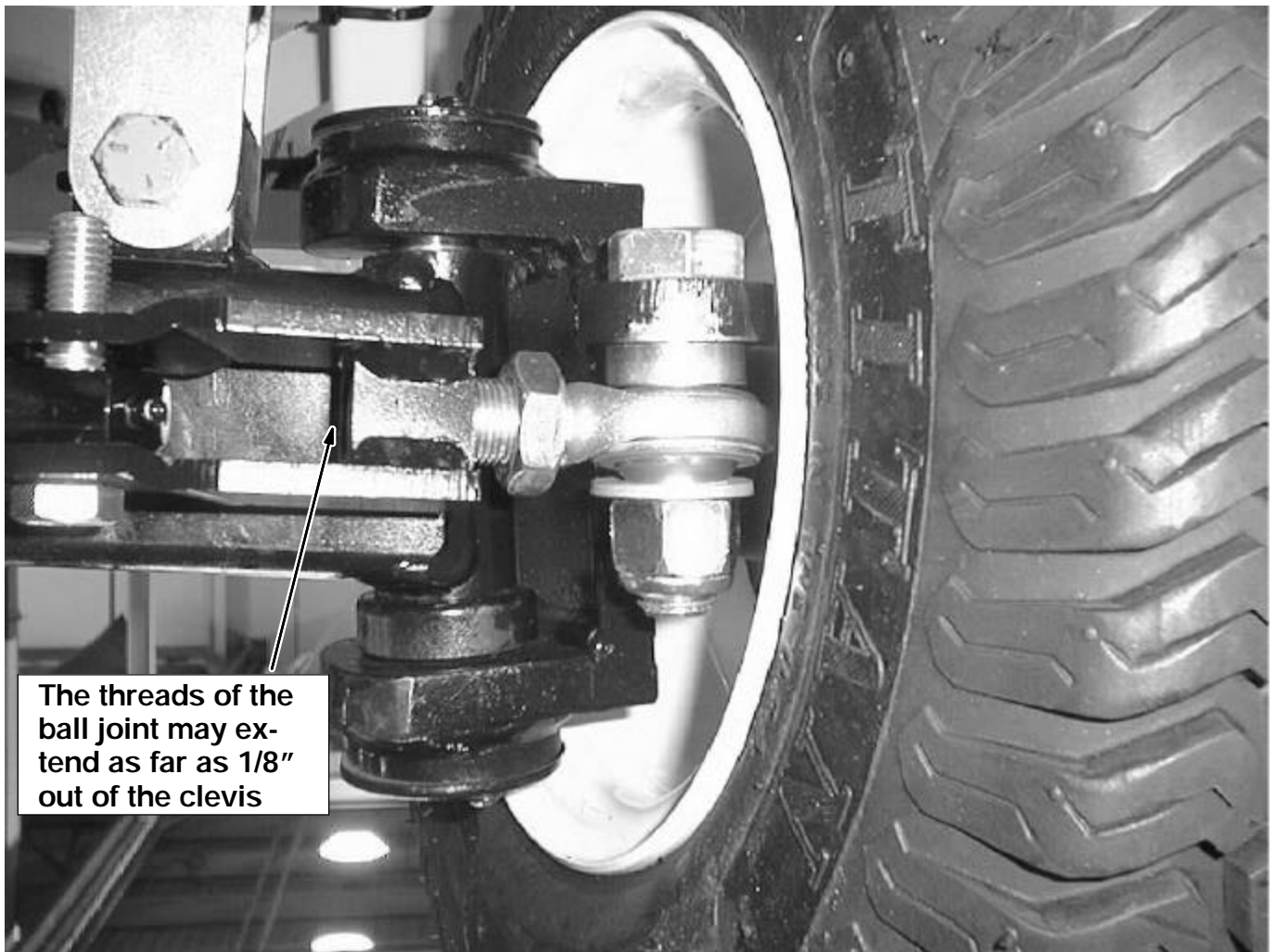
FIG. 5 BALL JOINT ADJUSTMENT
